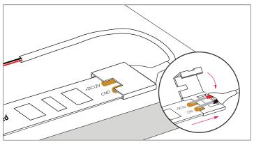
4 Our \*Strip Connector enables quick, solder-free joining of wires or LED strips. Various connector types are available to suit specific applications (see Figure 2, page 2).
