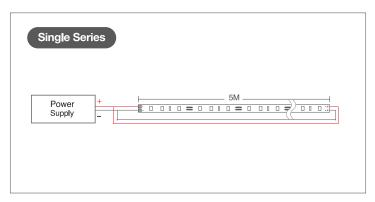
Do not exceed the maximum length of LED strips per series (**refer to each item's spec sheet**). We recommend wiring both ends of LED strips to the power supply.
