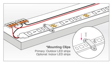
WAGO connectors enable quick wiring of LEDs in series. Use mounting clips and screws that match the width of the strip to support the LED strip light.
