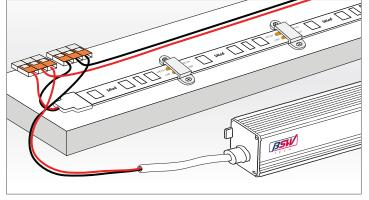
6 Wire both ends of LED strips to the power supply. For multiple series, connect them in parallel to avoid voltage drop and ensure brightness. (refer to Figure 3 on page 2)
