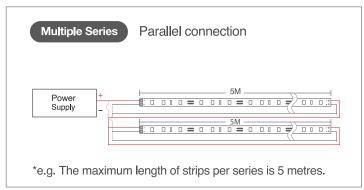
If you require **multiple strips**, they must be wired in parallel as a safe electrical operation mode. **Serial connection is not recommended**, as unbalanced voltage drops can lead to hazardous overload, potentially damaging the LED strips and causing uneven brightness.
