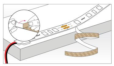
**3** Remove the adhesive tape, position the LED strips carefully, ensuring they are straight, and press firmly. Avoid removing and reapplying the strip (see Figure 1 on page 2).
